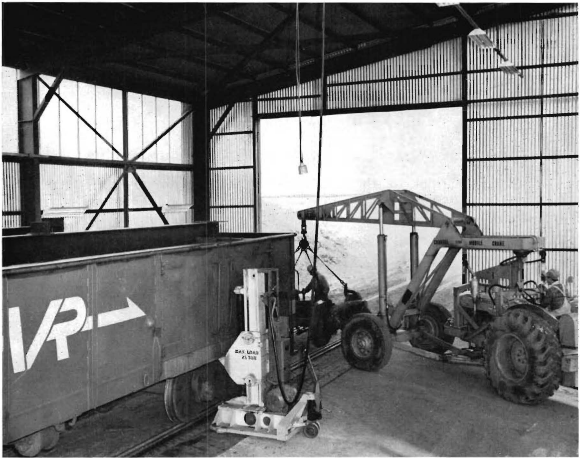
A bogie being placed in position by a mobile crane at the Bogie Exchange Centre.
