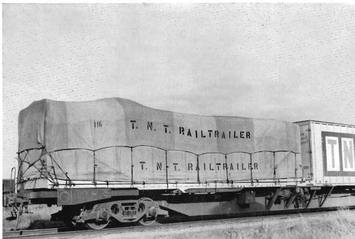
'Flexi-Flat' unit on wagon specially built to carry 'Flexi-Vans' in pairs.
